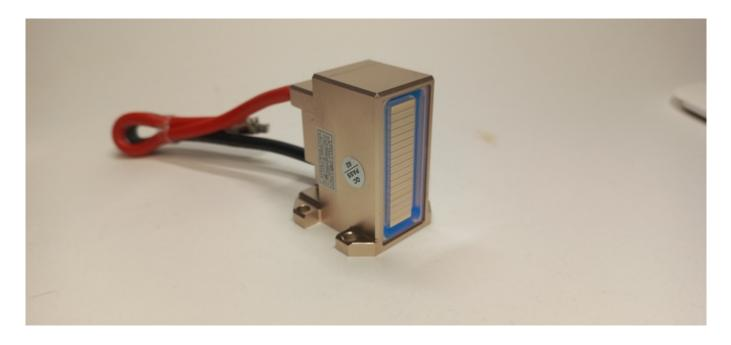
Drages in the work of the diode laser handle are expressed as follows: there is a loss of flashes and sensations.Damage can be detected visually through the transparent part of the handle.
