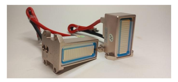
The main reason for the breakdown of the diode laser handle is the flashes stop and the sensation of tingling disappears. The handle defect is often visually observed through the window.
