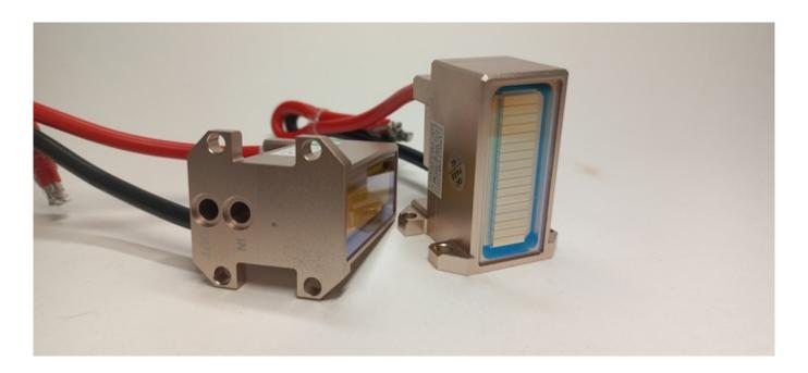
The main defect in the work of a diode handle is that there are no visual outbreaks and sensations on the skin. Often the problem is determined visually through the window on the handle.
