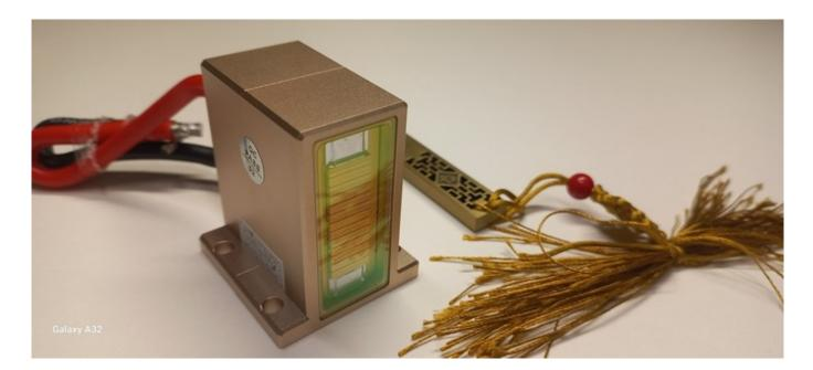
Often, the diode laser has a problem: the flashes stop and the sensation of tingling disappears.Damage can be detected visually through the transparent part of the handle.
