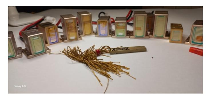
One of the typical problems of the diode laser is that flashes disappear and there is no tingling. Damage can be detected visually through the transparent part of the handle.
