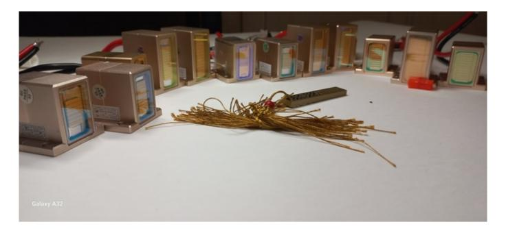
The main defect in the work of the diode handle is that the outbreaks do not occur, there is no tingling either.Damage can be detected visually through the transparent part of the handle.
