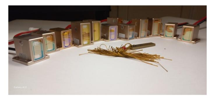
The main defect in the work of the diode handle is that flashes disappear and there is no tingling. Damage can be detected visually through the transparent part of the handle.
