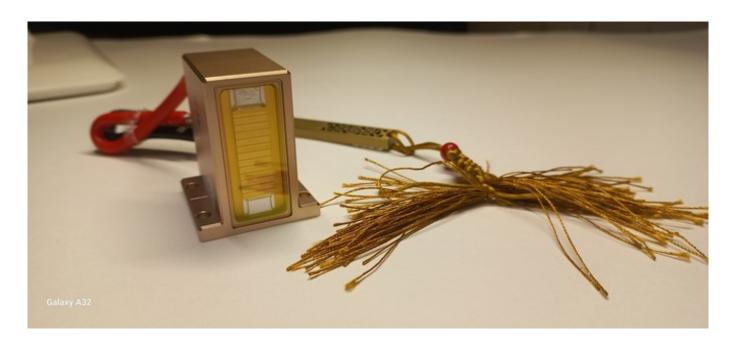
Frequent malfunction of the laser handle - no light impulses are visible, there is no contact with the skin. Damage is often visible through the observation glass.
