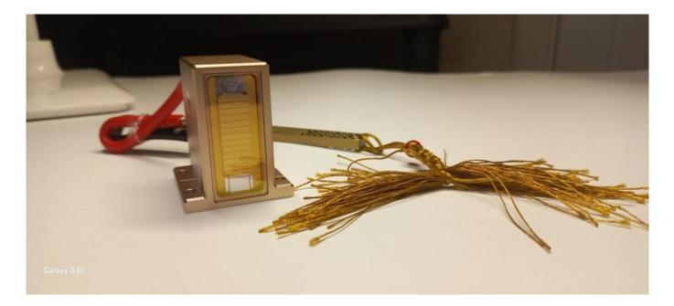
A common breakdown of the handle is that there is a loss of flashes and sensations. Through the observation window, the cause of the breakdown is often visible.
