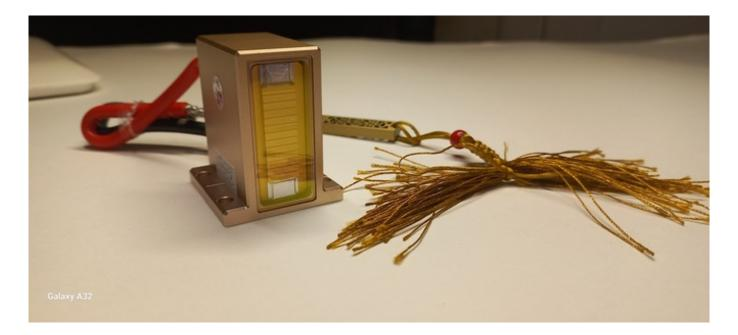
Frequent malfunction of the laser handle - impulses do not pass, the patient does not feel tingling.Damage can be detected visually through the transparent part of the handle.
