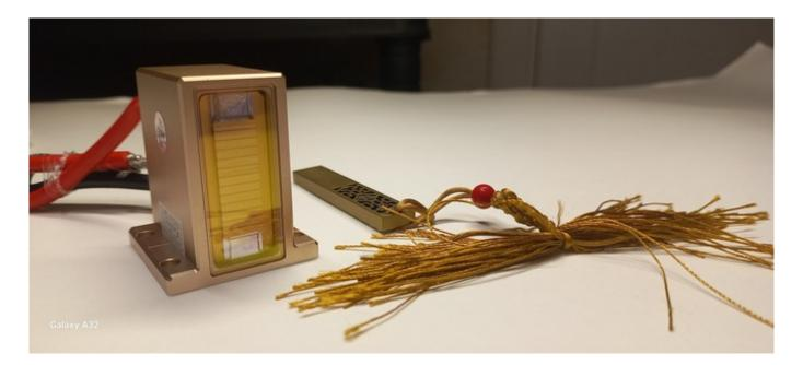
The main reason for the breakdown of the diode laser handle is no light pulses, there is no contact with the skin. Through the observation window, the cause of the breakdown is often visible.
