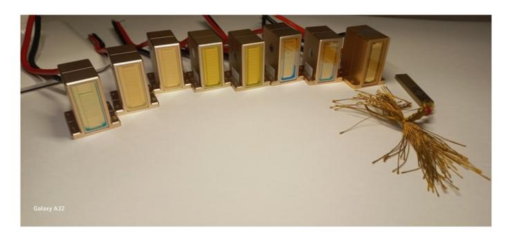
The main defect in the work of a diode handle is that the laser does not emit flashes and does not cause sensations. Damage can be detected visually through the transparent part of the handle.
