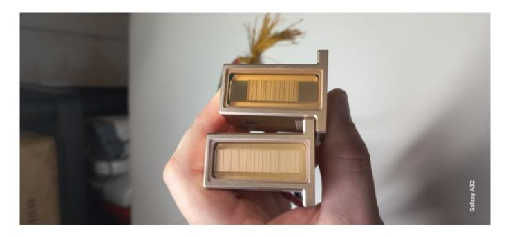
The main reason for the breakdown of the diode laser handle is that flashes disappear and there is no tingling. The breakdown is often noticeable when examining the handle.
