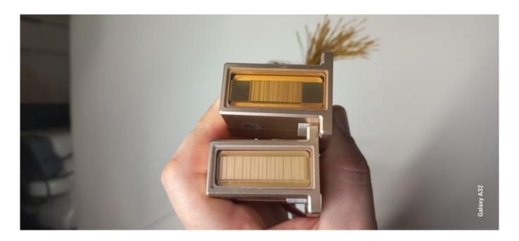
Often, the diode laser has a problem: there are no visual outbreaks and sensations on the skin. The handle defect is often visually observed through the window.
