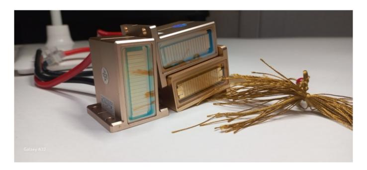
Often, the diode laser handle fails: the laser does not work, and the sensations disappear. Damage can be detected visually through the transparent part of the handle.
