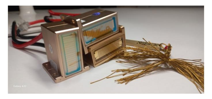
One of the typical problems of the diode laser is that the laser does not work, and the sensations disappear. Damage is often visible through the observation glass.
