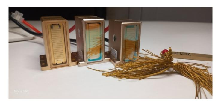
Often, the diode laser has a problem: there are no visual outbreaks and sensations on the skin. Through the observation window, the cause of the breakdown is often visible.
