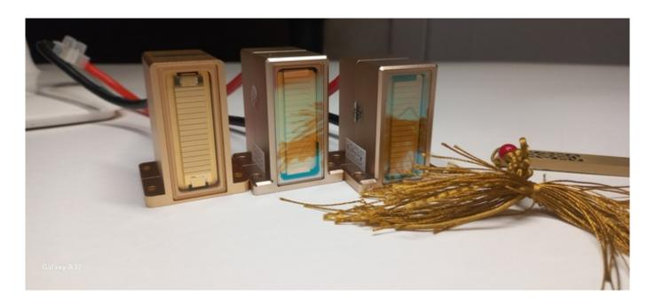
Often, the diode laser handle fails: the laser ceases to give out impulses, there are no sensations. Often the problem is determined visually through the window on the handle.
