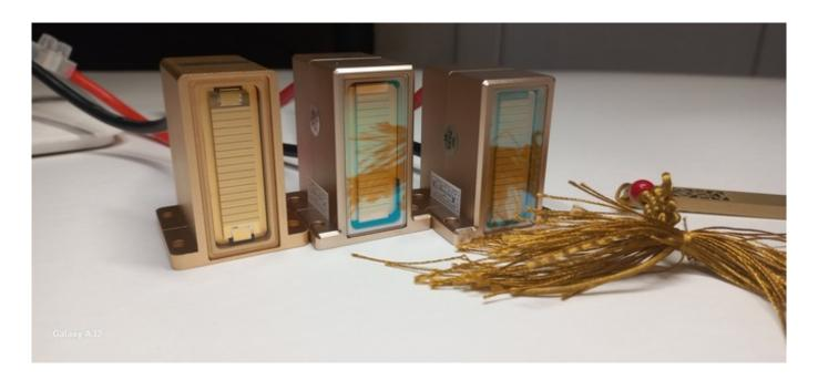
Often, the diode laser handle fails: no light impulses are visible, there is no contact with the skin. Often the problem is determined visually through the window on the handle.
