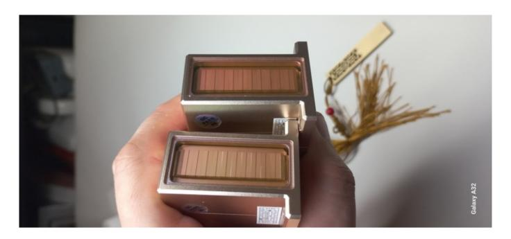
A common breakdown of the handle is that flashes disappear and there is no tingling. Damage is often visible through the observation glass.
