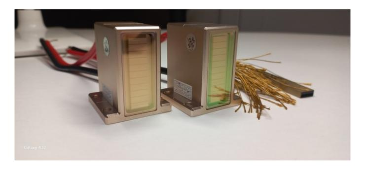
The most common problem with the diode laser handle - the laser stops issuing impulses, there are no sensations. Damage can be detected visually through the transparent part of the handle.
