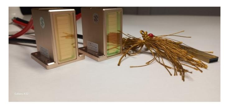
Often, the diode laser has a problem: the laser stops issuing impulses, there are no sensations. The handle defect is often visually observed through the window.
