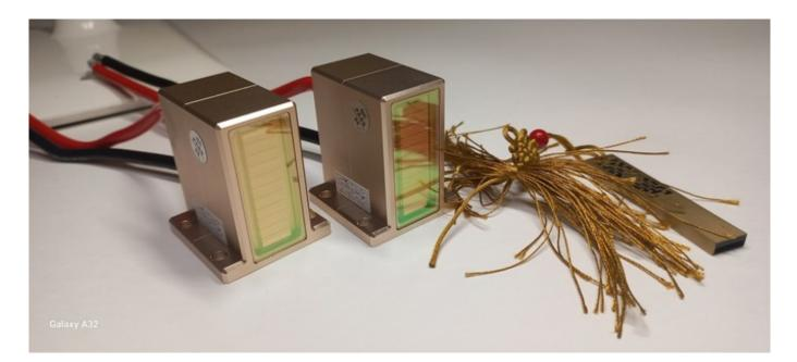
The most common problem with the diode laser handle - the laser stops issuing impulses, there are no sensations.Damage is often visible through the observation glass.
