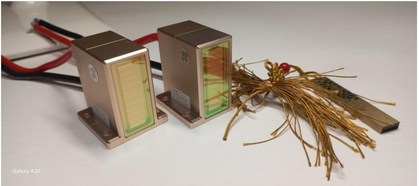
A common breakdown of the handle is that there are no light impulses, there is no contact with the skin. Through the observation window, the cause of the breakdown is often visible.
