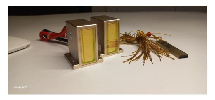
The main reason for the breakdown of the diode laser handle is the impulses do not pass, the patient does not feel tingling. The handle defect is often visually observed through the window.
