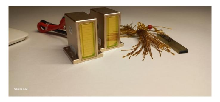
In most cases, the handle malfunction is due to the fact that the laser stops issuing impulses, there are no sensations. Often the problem can be seen through the observation window.
