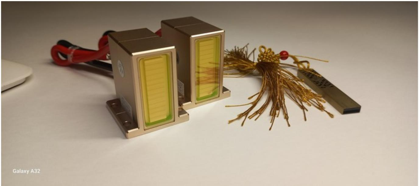
One of the typical problems of the diode laser is that the outbreaks stop and the sensation of tingling disappears. Often the problem is determined visually through the window on the handle.
