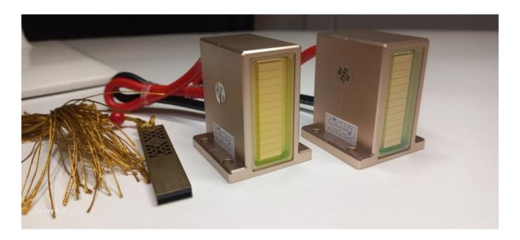
The most common problem with the diode laser handle - the laser stops issuing impulses, there are no sensations. Often the problem can be seen through the observation window.
