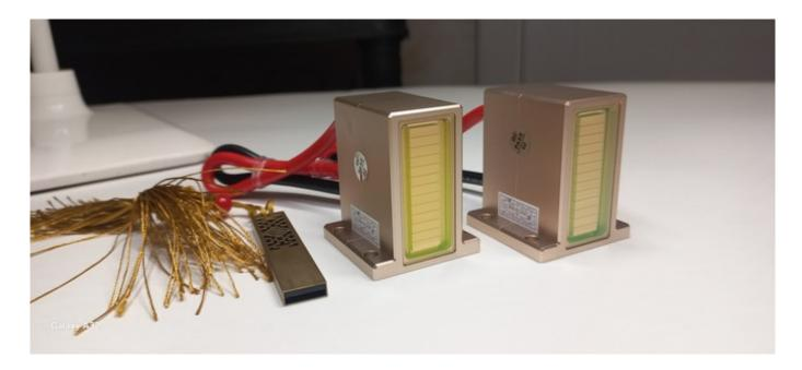
A common breakdown of the handle is that the laser does not emit flash and does not cause sensations. Often the problem can be seen through the observation window.
