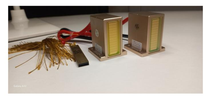
In most cases, the handle malfunction is due to the fact that flashes disappear and there is no tingling. Through the observation window, the cause of the breakdown is often visible.
