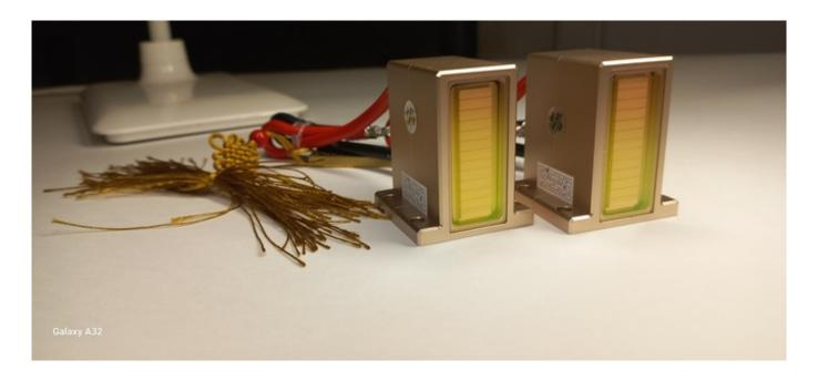
In most cases, the handle malfunction is due to the fact that there is a loss of flashes and sensations. Often the problem can be seen through the observation window.
