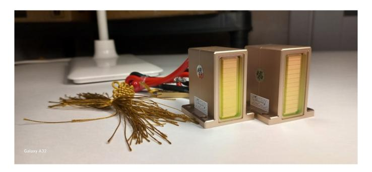
Often, the diode laser handle fails: the laser does not emit flash and does not cause sensations. Often the problem is determined visually through the window on the handle.
