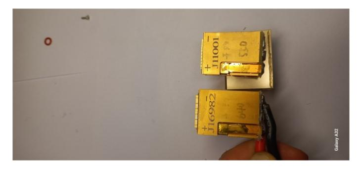
Components for replacing elements in the laser handle
