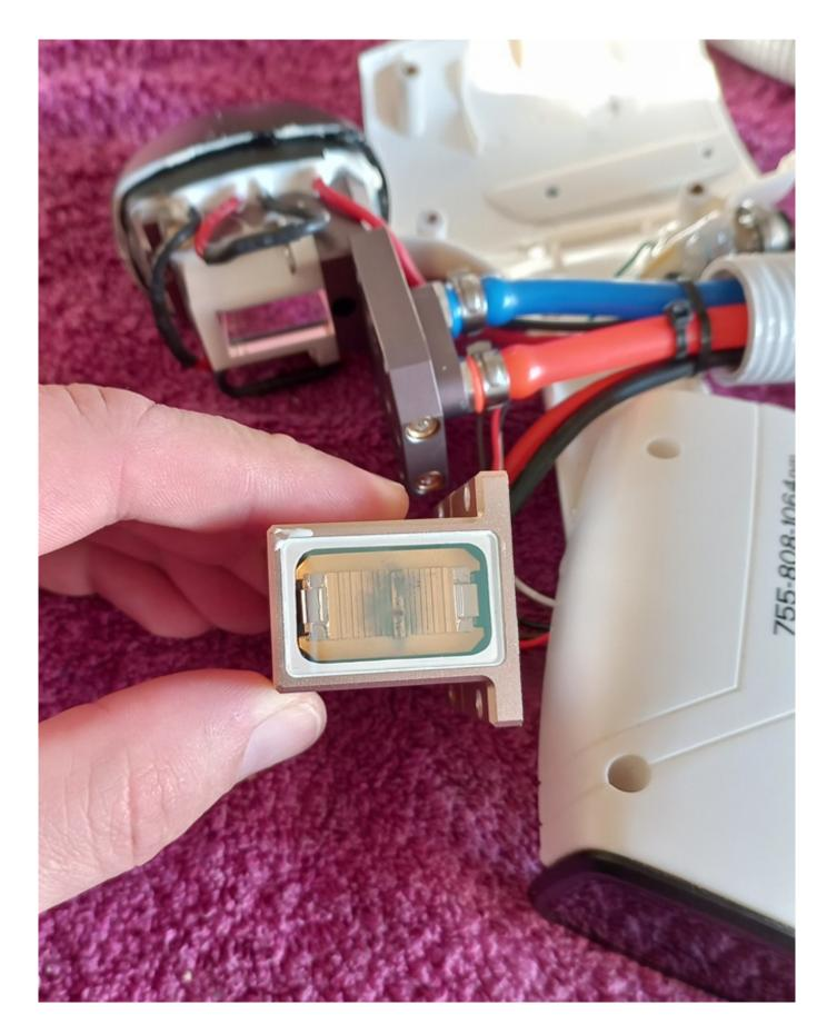
Exchange elements of a diode epilator manipules
