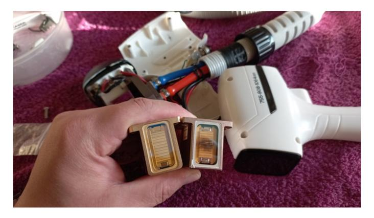
Spare parts for the manipula of aesthetic diode laser
