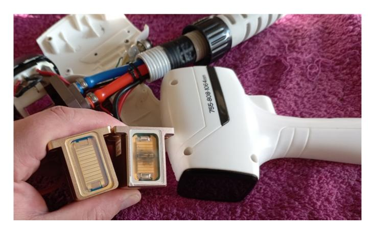
Elements for replacement in the manipul of the laser apparatus
