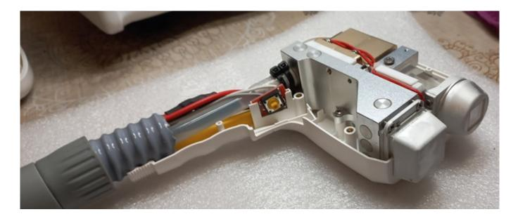
Diode laser manipula components for repairing
