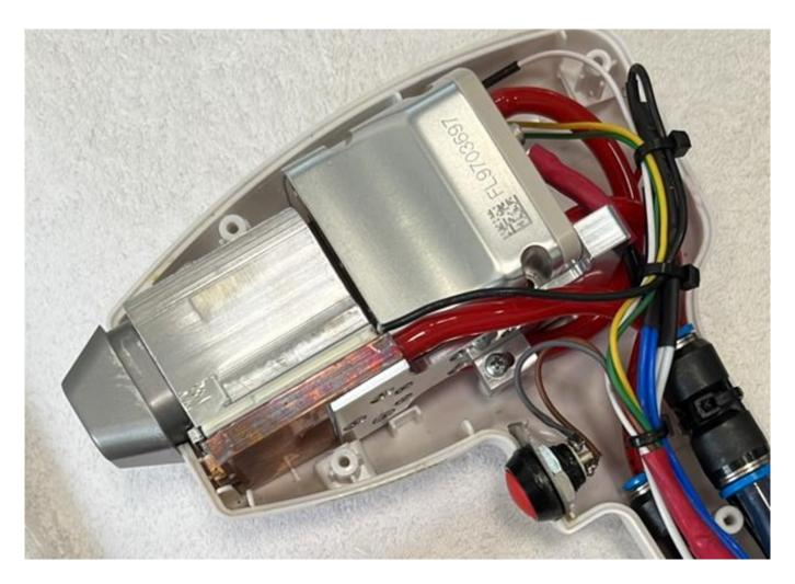
There are 808nm laser modules for diode devices.
