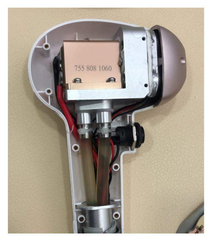
Reliable diodes 808nm: capacity choice from 200 to 1600 watts.
