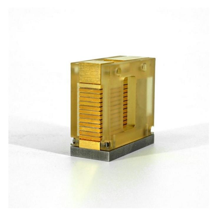
We put a 808nm diode module for your device.
