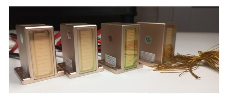
808nm diodes at capacities from 200 to 1600 watts are available.
