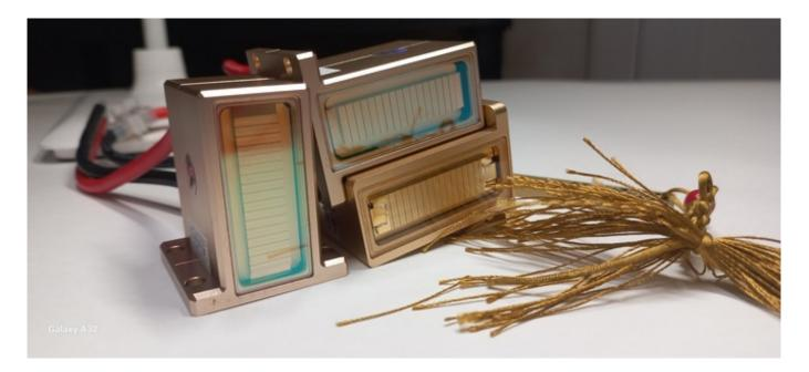
There are 808nm laser bars for 200-1600 watts.
