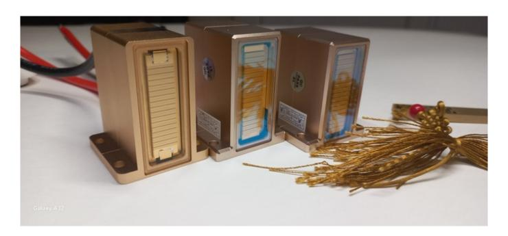
Diode stacks for replacement for lasers 808nm.
