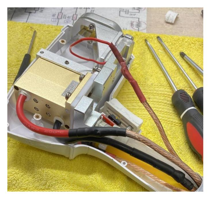
Installation of bars and repair of diode lasers manipuli 808nm.
