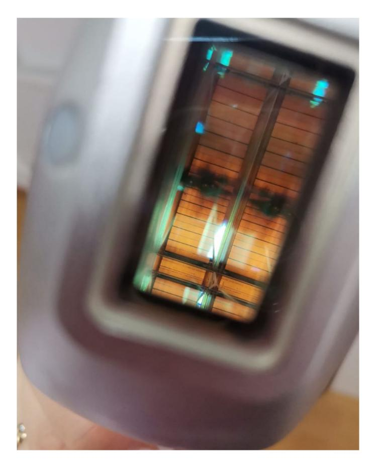
Setting up and repairing pens 808nm with bars replacement.
