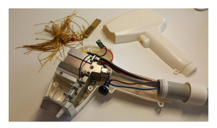
Fixing of laser handles 808nm with replacement of glasses and diodes.
