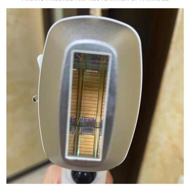
Restore the laser handle 808nm, set the bar of the desired power.
