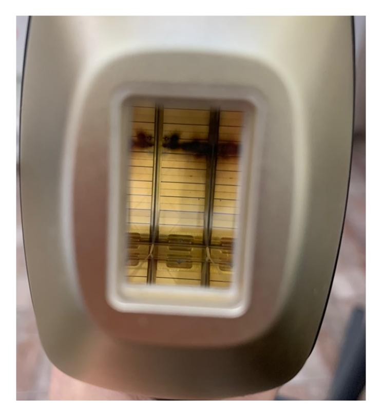
Replacing diodes in manipulas 808nm, elimination of problems.
