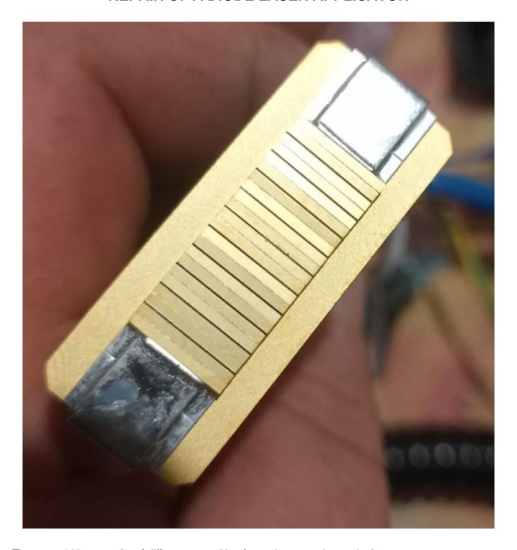
There are 808nm stacks of different capacities for replacement in manipulas.
