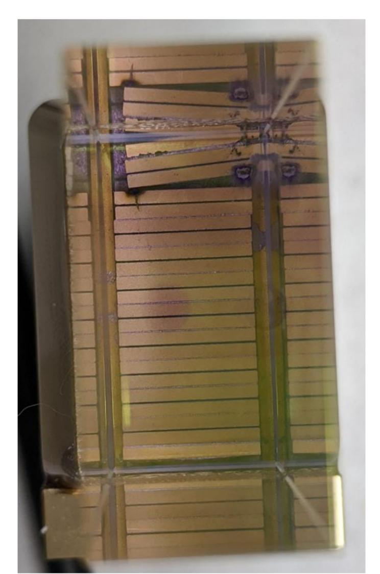
Repair and modernization of laser manipules under 808nm diodes.
